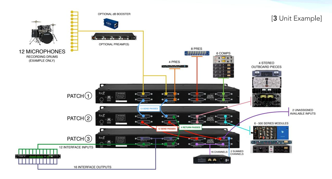
Optional Addition of a Clean dB Booster (**Mic > dB Booster > PATCH**) is recommended with some microphones (I.E. Dynamic Mic's) to achieve better initial signal input level prior to PATCH. In some cases a low output Condenser Mic may require a Preamp to be placed before PATCH.
